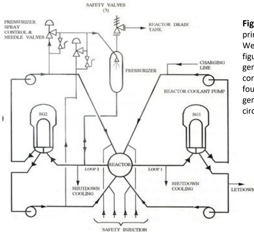
**Figure 5:** Schematic of the primary coolant circuit of a Westinghouse PWR. The figure shows two steam generators for the single core. Diablo Canyon has four parallel steam generator (SG1 and SG2) circuits.
