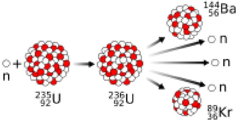
**Figure 2:** Schematic of the fissioning of  $^{235}\text{U}_{92}$  by slow neutrons.
