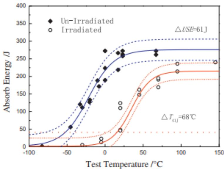
**Figure 4:** Effect of neutron irradiation on the Charpy impact test results for a fluence of  $10^{20}$   $\text{n/cm}^2$  ( $E > 1$  MeV) for A508-3 RPV steel. After Lin, et.al.
