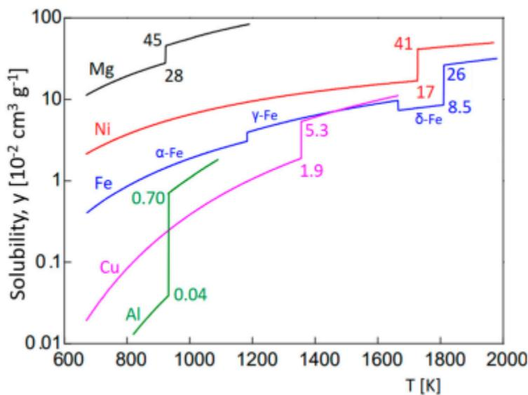
**Figure 7:** Solubility of hydrogen in various metals as a function of temperature, after Z. Weiss<sup>38</sup>.
