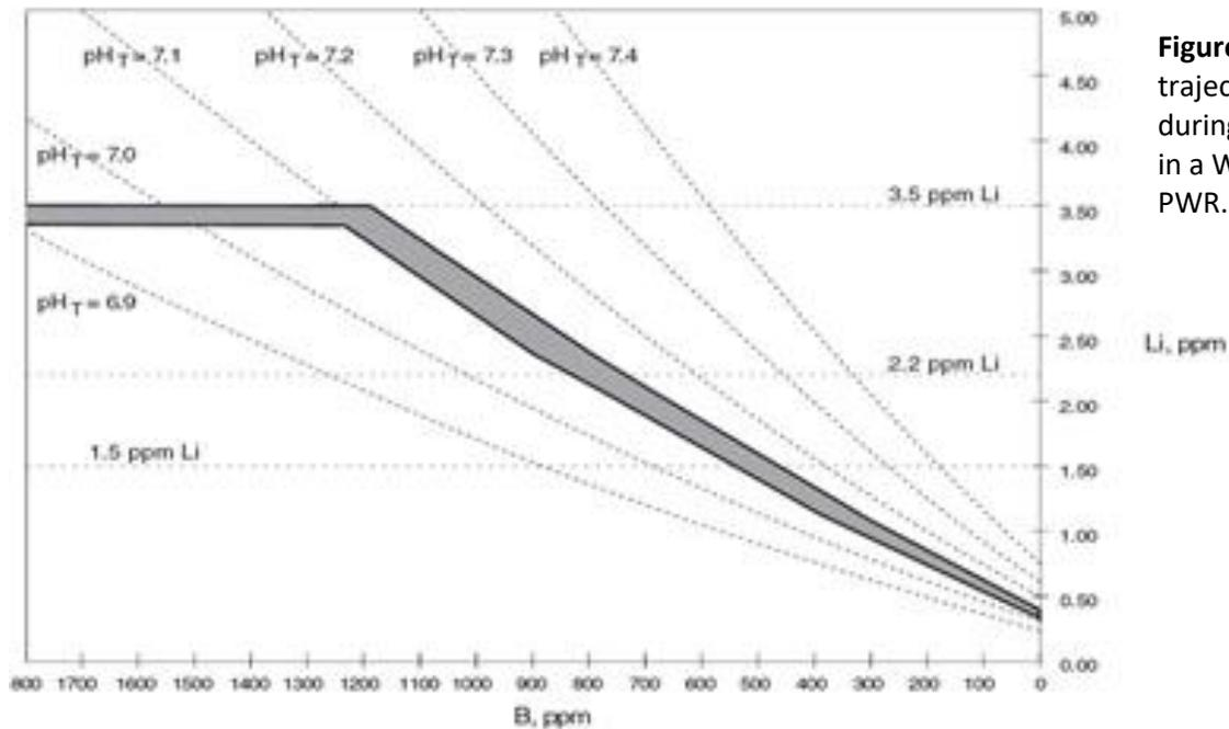
**Figure 6:** Desired trajectory of pH during fuel burn-up in a Westinghouse PWR.
