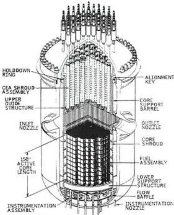
**Figure 1:** Cut-away schematic of the core of a typical pressurized water reactor (PWR).
